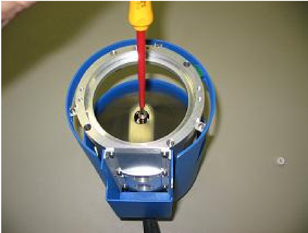
Figure 2. Removing the securing nut
