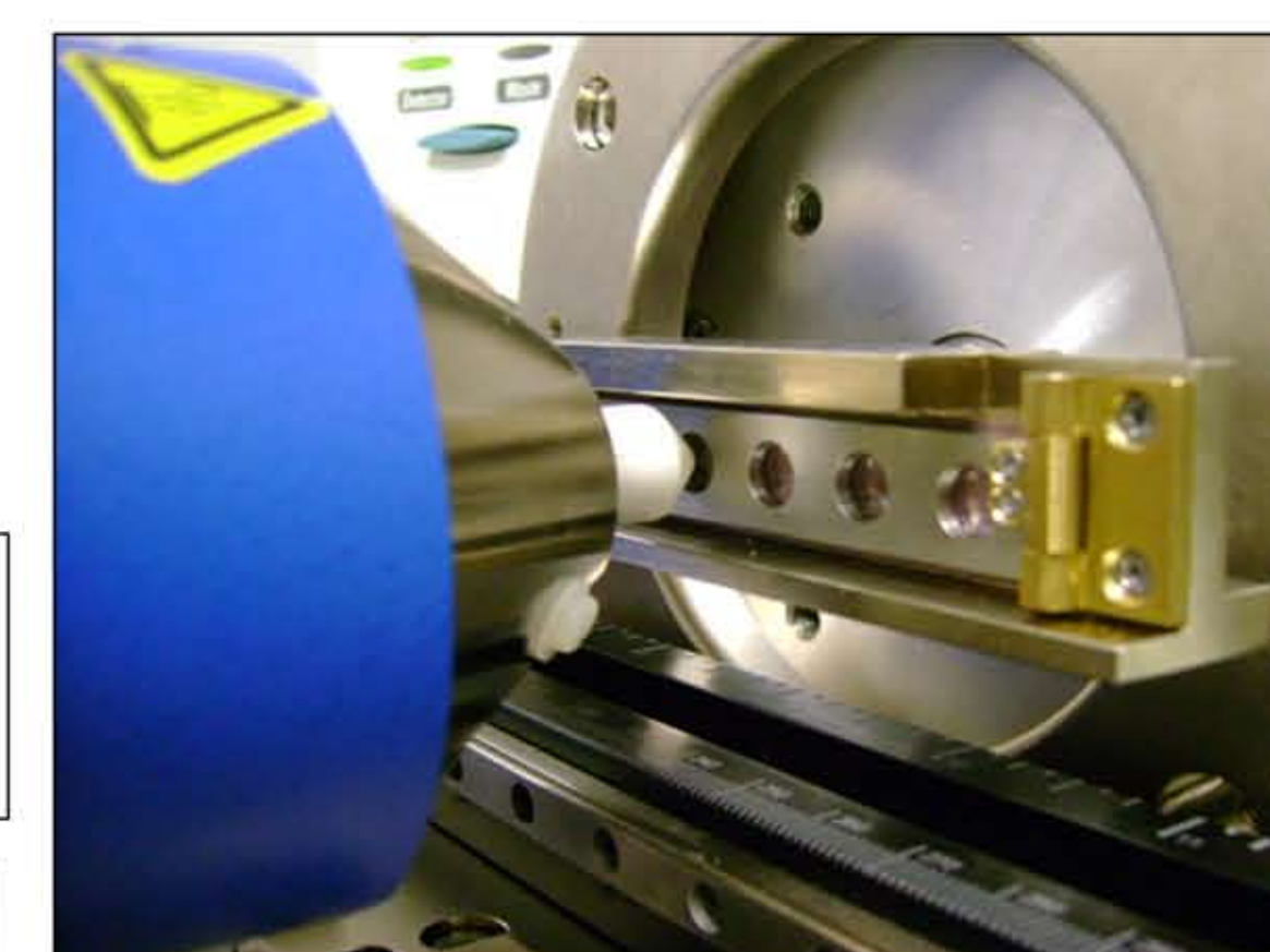
Figure 2. 1-D transmission module mounted for DART analysis. Typical analysis speed is 0.5 - 1.0 mm/s through the DART ionization region.
