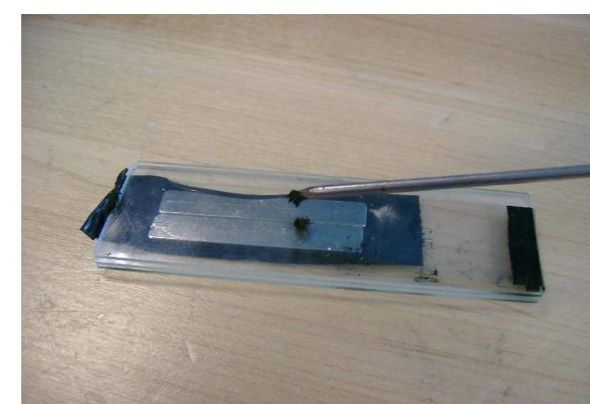
Figure 3: Metal powder is transferred to the glass slide with a magnetic micropipette and held in place by the neodymium magnet underneath.
